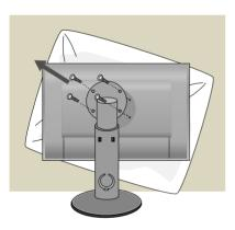
**2.** Separate the head and the stand with the use of a screwdriver.
